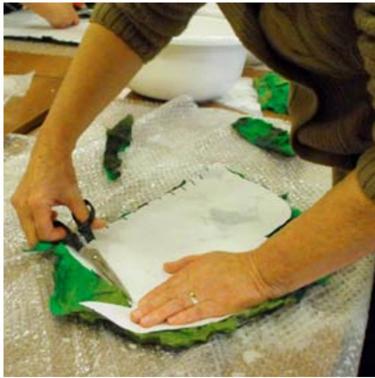
Above - A piece of green pre-felt is cut to the required shape using a paper template.
